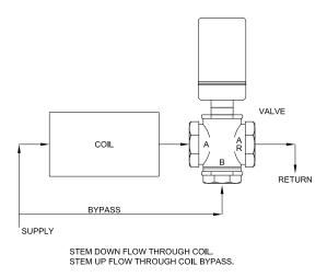
3. When the demand is satisfied, the limit operating circuit opens and the valve actuator is de-energized. The actuator motor stops running and the actuator shaft spring returns to the retracted position causing the boiler water to divert through the bypass ports and return to the boiler water supply loop.
